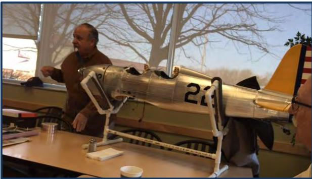
Phil used pieces of aluminum furnace tape to simulate aluminum panels to cover this typically fabric trainer. He also simulated a full rivet pattern. The attention to detail was very impressive, as these photos confirm.
