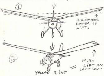
in flight. As you can see, both wings are level and meeting the air at the same angle of attack. In DRAWING #2 the aircraft has been yawed to the right with rudder. This forces the left wing out ahead of the right wing and also increases the angle of attack of the left wing. This in turn increases the lift of the left wing and causes the plane to bank to the right in the direction the rudder was applied. The result is a banked right turn without ailerons!
