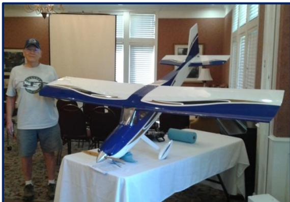
This handsome high-wing was fitted with a Rimfire 1.60 and powered by two 4S Lipo batteries, which should provide plenty of power. The flaps were operational, and Bill opted to keep the taildragger configuration over the optional tripod.
