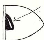
BE SURE PROPIS NOT TOUCHING SPINNER CUT OUT TO PREVENT BLADE FAILURE.
