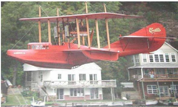
The original aircraft had a 72' wingspan. In 2008 a full size reproduction of the "America" was completed by the Glenn H Curtis Museum. It was "water tested", but I'm not sure if it was flown. It was powered with two 120 hp OXX-6 engines.
