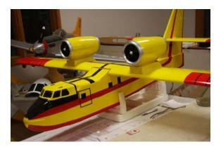
I got the idea for this "jet" conversion from the Russian Be-200 water bomber. The jet pods and 100 mm fans are from my crashed Nitroplanes Citation jet. The wing mounting blocks are the bottom 1/3 of the original motor mounting blocks. I simply ran them thru the band saw, and covered them with balsa and Monokote
