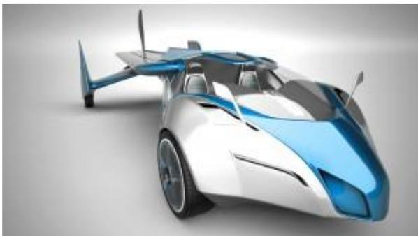
The top of the page shows the Aeromobil with wings out. The Rotax 912 powered car will supposedly fit in a standard parking space, and burn regular gas.
