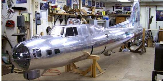
The faux B-17 is a remarkably accurate replica externally, and Bally can think of few compromises he's had to make. "The gear-retraction mechanism is hydraulic and not through jackscrews, and the engines aren't radials,"
