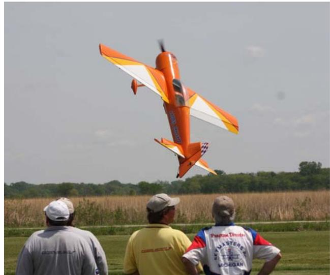
As you might recall, most of their aircraft were powered by DA-150's, 150 cc motors. The wingspans of the aircraft were about 120 inches. Shown above is a Yak-54 doing a 3-D maneuver., and flown by Phil Eason.
