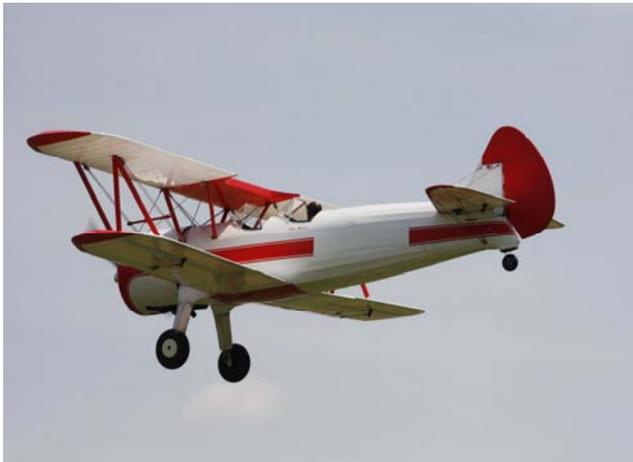
Here is the big "18" in a bank prior to landing. The craft weighs about 45 lbs. and has a 114" wingspan.
