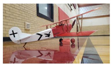
This is a 2004 Sig park flyer Fokker D7, it has a 180 brushed motor with a 4 to1 gear reduction. 32-in wingspan and 8 oz is all up weight. Testing continues. . .
