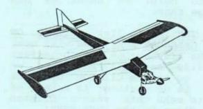
Wing Span: 52" Wing Area: 585 Sq In Weight: 3-1/2 to 4 Lbs Length: 41" Engine: .30-.45 2 Cycle
