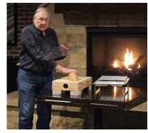
Keep it in there until the plastic just starts to sag. The next piece to build is the vacuum box. You want your shop vac running when you pull the plastic out of the oven and place on the mold. Made mold out of Styrofoam and shaped it and used bondo to fill in any gaps. (His was brown, so I might have missed a step here). Bought 30/1000 plastic on Amazon. Got TG (did not catch the entire name). For window sides, you can probably use your heat gun to heat the plastic.
