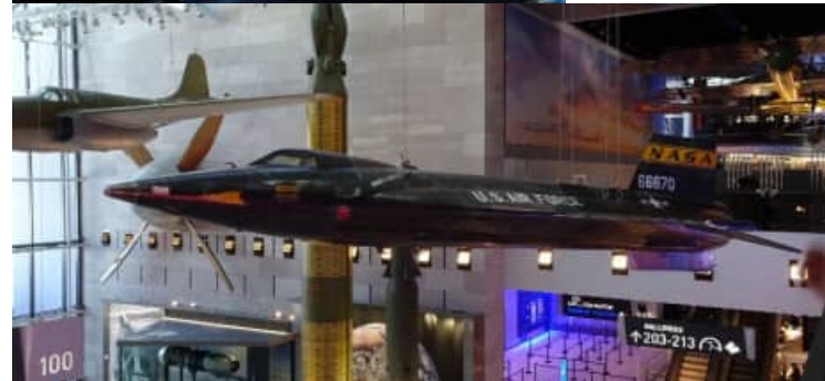
North American X-15 rocket plane: 4,000+ mph, Mach 6+, 50-60 mile altitude. Seems like they don't make'em like that anymore!
